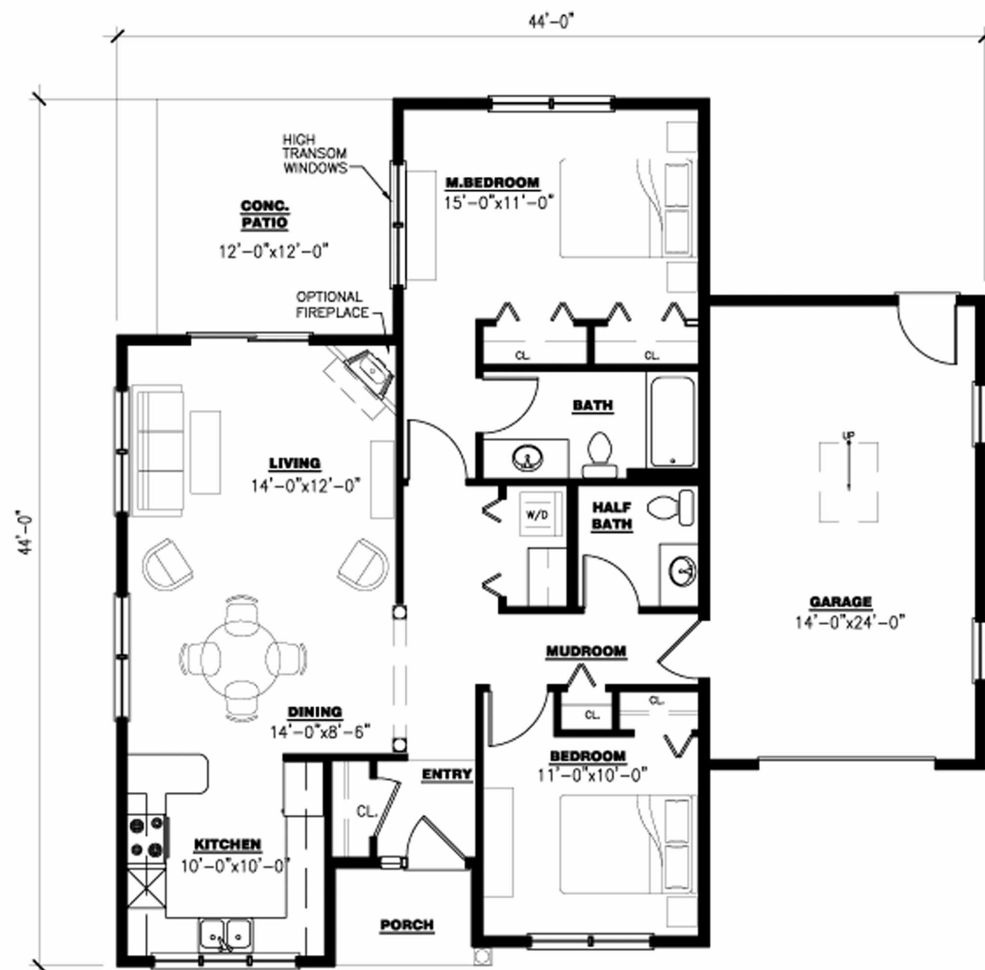
FIRST FLOOR PLAN -CARRABASSETT N.T.S. 1,105 S.F.
