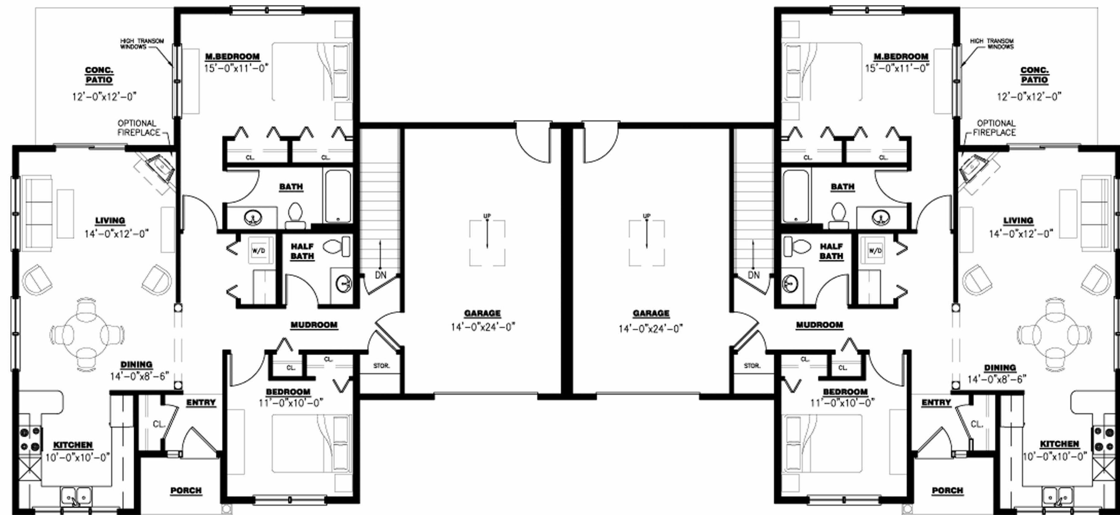
FIRST FLOOR PLAN -DUPLEX W/BASEMENT OPTION N.T.S. 1,198 S.F.
